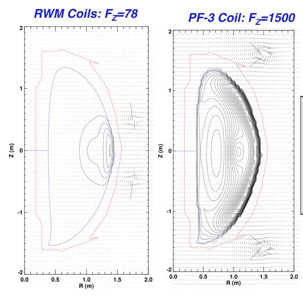
*RWM Coils make far less force for the same power supply current.*
